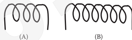
FIGURE 10.78 (A) Few turns, low inductance; (B) more turns, higher inductance.
