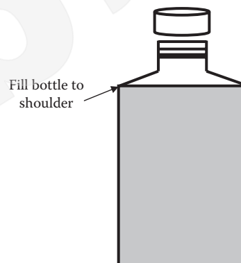
FIGURE 17.12 Sampling bottle. Filling to the shoulder ensures collecting enough sample—do not overfill.
