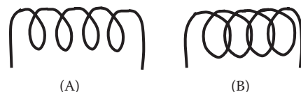
FIGURE 10.79 (A) Wide spacing between turns, low inductance; (B) close spacing between turns, higher inductance.
