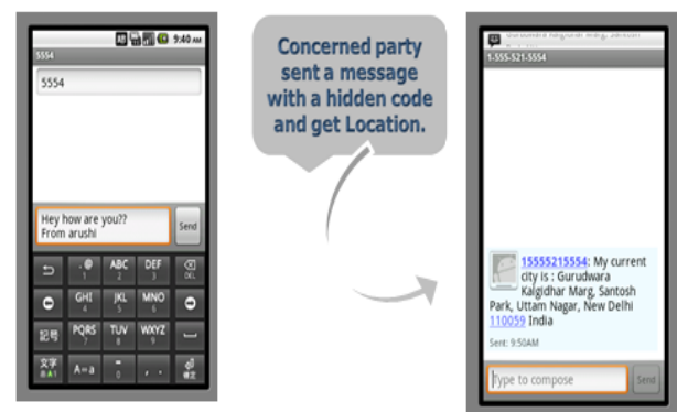
Fig 1. Example of Tracking the Location through SMS The figure shown above depicts that when 5558 emulator has text 5554 (as in left side emulator), the application has detected the code and automatically sent the second party location to the concerned party which is 5556 in this case (as in right side emulator).
