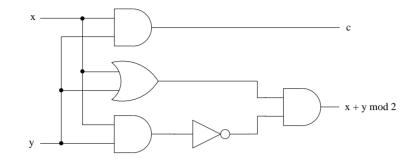
Fig. 4.7. Half-adder circuit as an example for a Boolean network.
