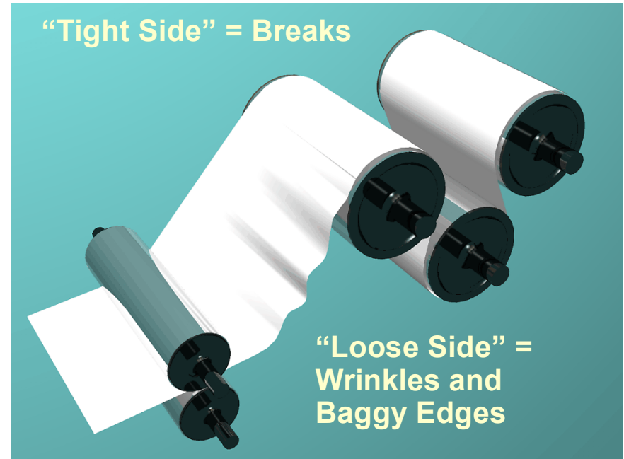
Figure 19: Effects of misalignment on web processes.
