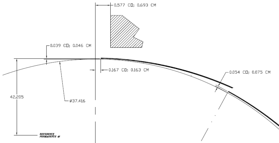
Figure 14: Ballistic jet geometry of paper machine headbox.
