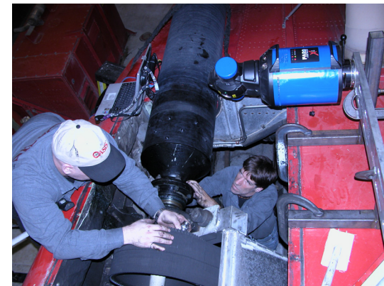
Figure 15: OASIS Engineers use a laser tracker to align drive components.
