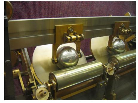
Fig. 9 Harmonic analyzer disc and sphere (Andy Dingley))
