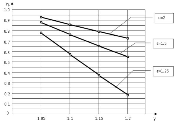
Figure 14. Relative efficiencies of the valve-less engine
