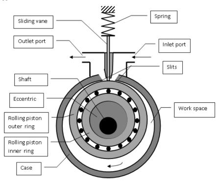
Figure 10. Valve-less rolling piston expander
