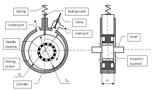
Figure 2. One-valve rolling piston expander
