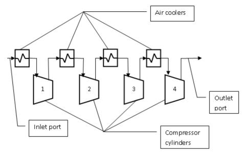
Figure 7. Air pass in a multi-cylinder compressor
