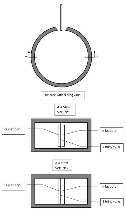
Figure 12. Two versions of the valve-less rolling piston heat engine design
