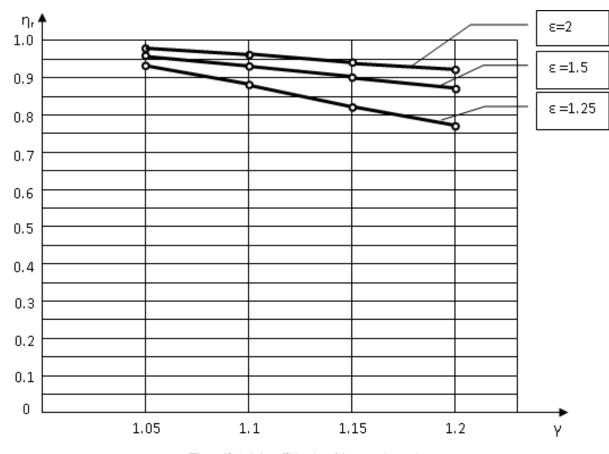
Figure 13. Relative efficiencies of the one-valve engine
