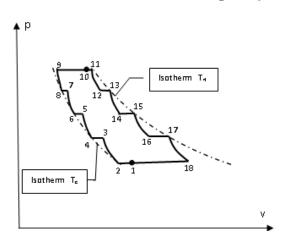
Figure 9. p-v diagram of the multi-cylinder 1-valve heat engine
