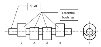
Figure 5. Shaft for a 4 cylinder expander/compressor
