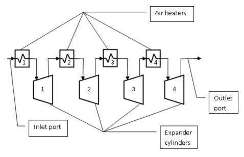
Figure 6. Air pass in a multi-cylinder expander
