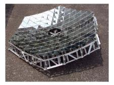
Figure 1. Solar concentrator prototype
