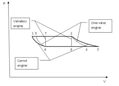
Figure 11. p-v diagram for three types of rolling piston heat engines: Carnot heat engine, one-valve heat engine, and valve-less heat engine
