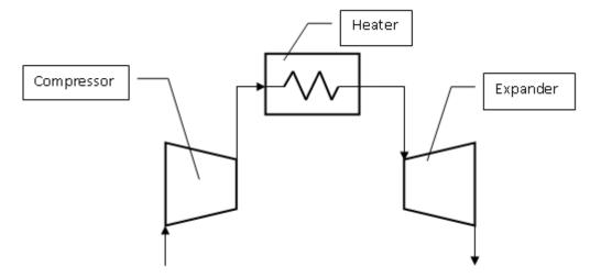
Figure 3. The simplest heat engine
