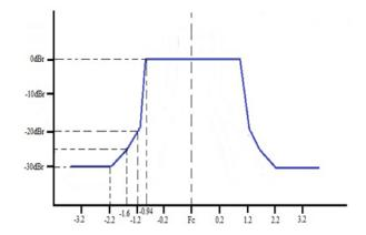
Figure 3. IEEE 802.11ad Spectral Mask measured with 100 kHz resolution bandwidth and 30 kHz video bandwidth
