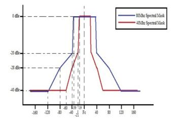
**Figure 4.** IEEE 802.11ac Spectral Mask for 40 MHz & 80MHz measured with 100 kHz resolution bandwidth and 30 kHz video bandwidth
