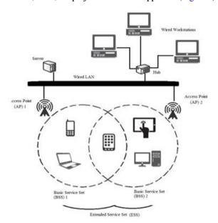
Figure 1. WLAN Network Architecture
