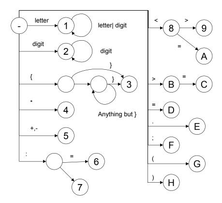
This FA handles only a subset of all Pascal tokens but it should give you an idea of how an FA can be used to drive a scanner. The numbered/lettered states are final states. The loops on states 1 and 2 continue to execute until a character other than a letter or digit is read. For example, when scanning "temp := temp + 1;" it would report the first token at final state 1 after reading the ":" having recognized the lexeme "temp" as an identifier token.
