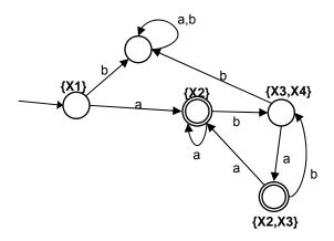
The process then goes like this: from a regular expression for a token, we construct an NFA that recognizes them using Thompson's algorithm. NFAs are not useful as drivers for programs because non-determinism implies choices and thus, expensive exhaustive backtracking algorithms. So, we use subset construction to convert that NFA to a DFA. Once we have the DFA, we can use it as the basis for an efficient non-backtracking scanner.
