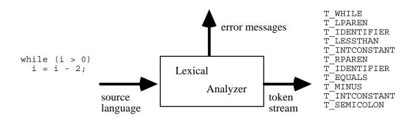
The lexical analyzer takes a source program as input, and produces a stream of tokens as output. The lexical analyzer might recognize particular instances of tokens such as:
