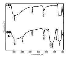
Figure 2. FT-IR spectra of (a) magnetic nanoparticles  $Fe_3O_4$ , (b) MNPs-MSA
