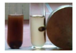
**Figure 5.** Image showing MNPs-MSA can be separated by applied magnetic field. A reaction mixture in the absence (left) or presence of a magnetic field (right)
