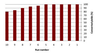
Figure 4. The recycling experiment of MNPs-MSA (5 mg, 0.87 mol %) in synthesis of 2-phenyl (amino) and phenyl (indolyl) kojic acid at room temperature
