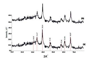
Figure 1. XRD patterns of MNPs (a) and MNPs@MSA (b)
