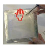
When using Amersham ECL Plex, avoid marking the membrane with a ballpoint pen - mark your membrane by cutting a corner or by using a pencil.
