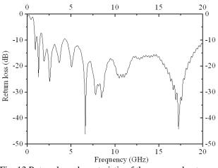
Fig. 13 Return loss characteristic of the proposed antenna with slot
