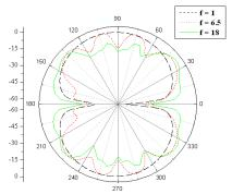
Fig. 6 Far field radiation pattern at frequencies 1 GHz, 6.5 GHz and 18 GHz for  $\theta = 90^{0}$
