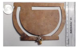
Fig. 14 Photograph of the fabricated SPQSMA
