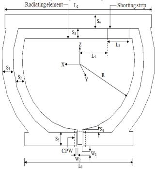
Fig. 1 Geometry of SPQSMA:  $L_1 = 96 \text{ mm}$ ,  $L_2 = 130 \text{ mm}$ ,  $L_3 = 25 \text{ mm}$ ,  $L_4 = 20 \text{ mm}$ ,  $W_1 = 4 \text{ mm}$ ,  $W_2 = 1 \text{ mm}$ ,  $S_1 = 10 \text{ mm}$ ,  $S_2 = 8 \text{ mm}$ ,  $S_3 = 8 \text{ mm}$ ,  $S_4 = 10 \text{ mm}$ ,  $S_5 = 10 \text{ mm}$ ,  $S_6 = 1.5 \text{ mm}$ , R = 50 mm
