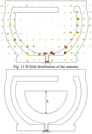
Fig. 12 Geometry of the proposed antenna with slot
