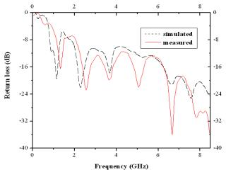
Fig. 15 Simulated and measured return loss characteristic of SPQSMA
