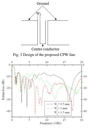
Fig. 4 Return loss characteristic of the antenna for different values of  $W_2$
