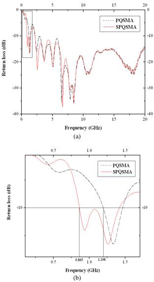
Fig. 2 (a) Simulated return loss vs. frequency of PQSMA and SPQSMA and (b) enlarged marked part of Fig. 2 (a)
