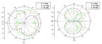
Fig. 5 Farfield radiation pattern at frequencies 1GHz, 6.5 GHz and 18 GHz for (a)  $\Phi = 0^{0}$  Pand (b)  $\Phi = 90^{0}$
