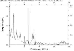
Fig. 9 Variation of group delay vs. frequency of SPQSMA The variation of phase response of the transfer function is
