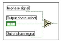
Figure 1-11. LabVIEW's Version of a Digital Data Selector
