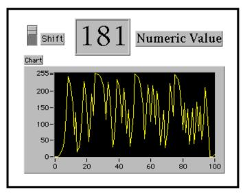
Figure 5-7. Numeric Output from an 8-Bit PRNG
