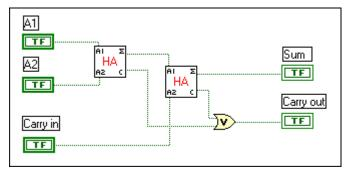
Figure 3-4. Full Adder Using Two Half Adder SubVIs
