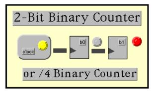
Figure 6-3. LabVIEW Simulation of a Divide-by-Four Binary Counter
