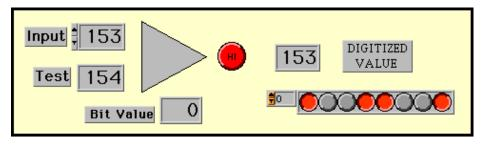
Figure 9-2. Digitized Value of an SAR ADC Displayed as a Boolean Array
