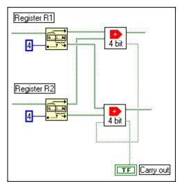
Figure 3-9. 8-Bit Adder Using Two 4-Bit Adders
