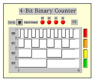
**Figure 6-5.** LabVIEW Simulation of a 4-Bit Binary Counter Observe the sequence and fill in the truth table below.
