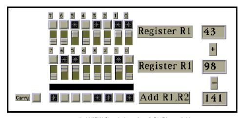
Figure 7-3. LabVIEW Simulation of an 8-Bit Binary Adder
