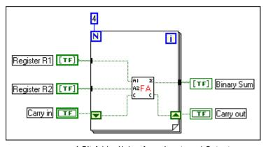
Figure 3-8. 4-Bit Adder Using Array Inputs and Outputs
