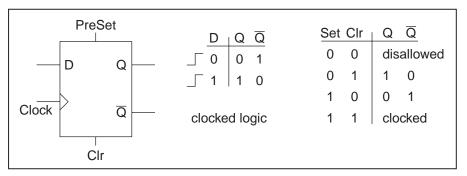
Figure 4-1. D-Latch Symbol and Truth Tables
