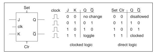
Figure 6-1. JK Flip-Flop Logic Symbol and Truth Tables
