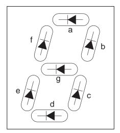
Figure 10-1. Seven-Segment Display Uses Seven LED Bars
