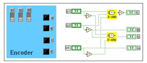
Figure 2-7. Encode.vi Front Panel and Block Diagram
