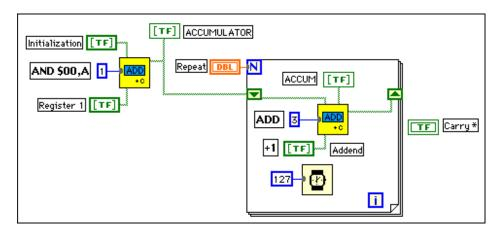
Figure 12-6. LabVIEW VI of an 8-Bit Binary Counter
