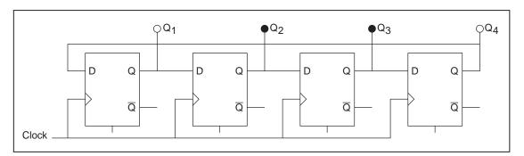
Figure 4-6. 4-Bit Ring Counter Using Integrated Circuit Chips
