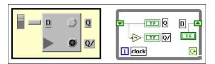
Figure 4-2. LabVIEW Simulation of a D-Latch
