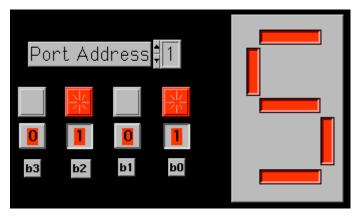
Figure 10-8. Binary-to-Seven-Segment Front Panel
