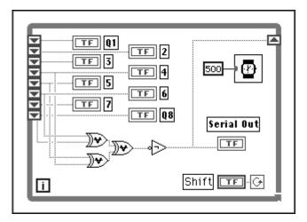
Figure 5-3. LabVIEW Simulation of an 8-Bit PRNG
