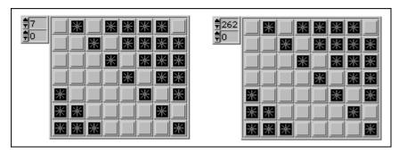
Figure 5-9. Boolean Array Representation of the 8-Bit Binary Pattern of the First Eight Numbers of an 8-Bit PRNG with the Patterns for Loops 262 to 268
