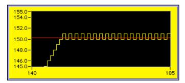
Figure 8-6. Tracking ADC Output when Input is Constant
