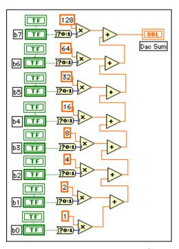
Figure 7-2. LabVIEW VI for 8-Bit DAC.vi
