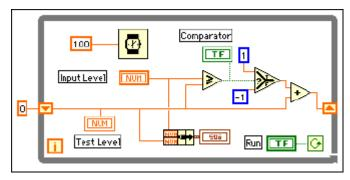
Figure 8-9. LabVIEW VI for the Tracking ADC
