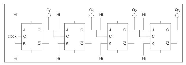
Figure 6-4. 4-Bit Binary Counter Built with JK Flip-Flops
