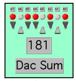
Figure 7-1. LabVIEW Simulation of an 8-Bit DAC
