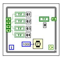
Figure 4-4. Block Diagram for an 8-Bit Shift Register
