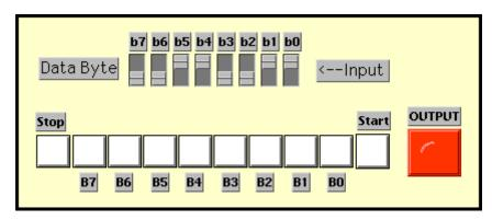
Figure 11-5. LabVIEW Simulation of a Serial Transmitter
