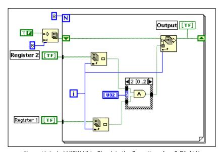
Figure 12-2. LabVIEW VI to Simulate the Operation of an 8-Bit ALU
