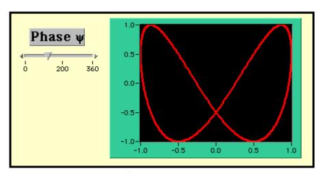
Figure 7-8. LabVIEW Simulation for a Lissajous Plot  $\omega_2=2^*\omega_1$
