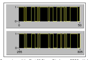
Figure 5-6. Comparison of the First 50 Binary Bits from a PRBS with Bits 255-305
