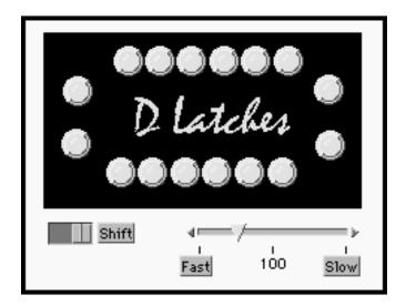
You can use the slide control to set the speed of the changing lights, and the 16 Boolean constants on the block diagram set the chase pattern.
