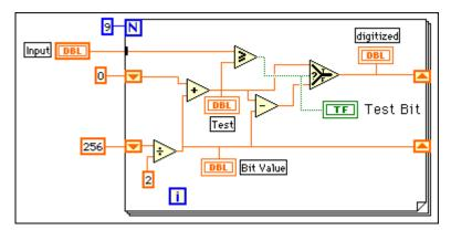
Figure 9-3. LabVIEW Simulation of the SAR Algorithm Using Shift Registers
