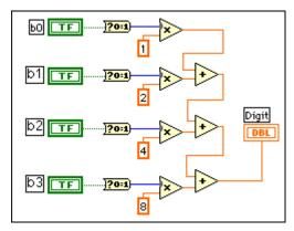
Figure 10-4. LabVIEW VI for a 4-Bit Digital-to Analog Converter
