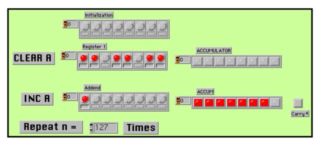
Figure 12-7. Front Panel for a LabVIEW Simulation of an 8-Bit Binary Counter
