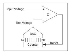
Figure 8-1. Symbolic Design for an 8-Bit Analog-to-Digital Converter
