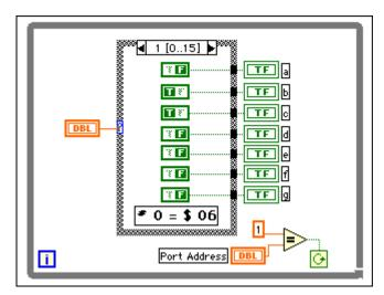
Figure 10-5. LabVIEW VI for Numeric-to-Seven-Segment Display
