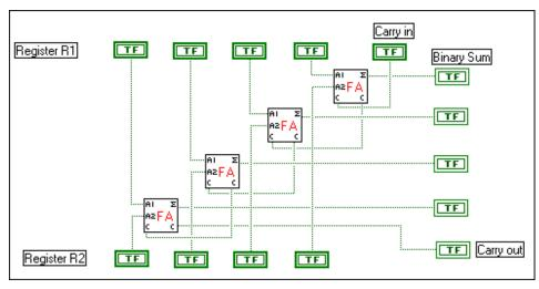
Figure 3-6. LabVIEW Block Diagram for 4-Bit Binary Addition
