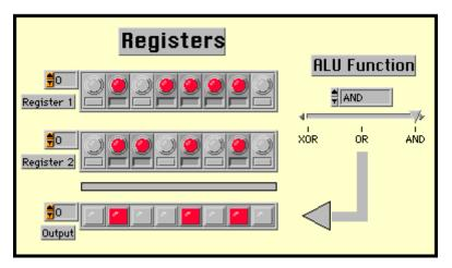
Figure 12-1. LabVIEW Simulation of an Arithmetic and Logic Unit
