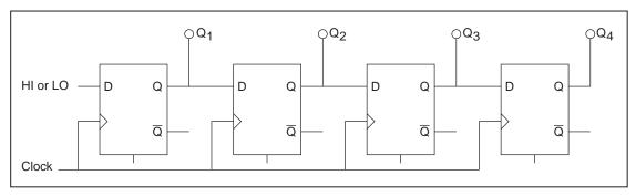
Figure 4-3. 4-Bit Shift Register
