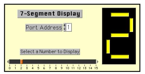
Figure 10-6. Hexadecimal-to-Seven-Segment Display Encoder and Indicator
