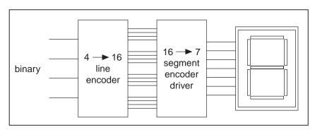
Figure 10-7. Symbolic Diagram of a Binary-to-Seven-Segment Display Circuit
