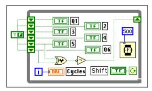
Figure 5-2. LabVIEW VI to Simulate a 6-Bit PRNG
