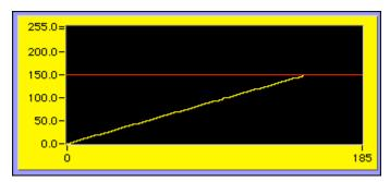
Figure 8-5. Tracking ADC Ramps Up to the Input Level Before Tracking Begins
