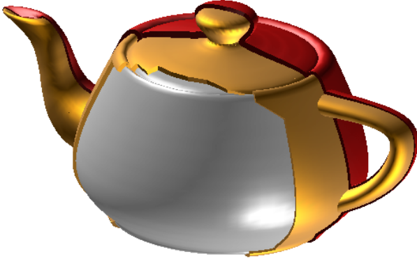
Fig 6.2: Middle surface and multiple layers of a shell: Inner surface and two layers are presented.
