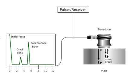
discontinuity (*such as a crack*) in the wave path, part of the energy will be reflected back from the flaw surface. The reflected wave signal is transformed into an electrical signal by the transducer and is displayed on a screen. Knowing the velocity of the waves, travel time can be directly related to the distance that the signal traveled. From the signal, information about the reflector location, size, orientation and other features can sometimes be gained.
