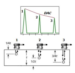
The same method is used for constructing DAC curves for <u>angle beam transducers</u>, however in that case both the <u>first and second leg reflections</u> can be used for constructing the DAC curve.
