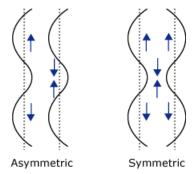
little motion occurs in the direction parallel to the plate. In this mode, the body of the plate bends as the two surfaces move in the same direction.
