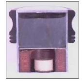
The <u>thickness of the active element</u> is determined by the desired frequency of the transducer. A thin wafer element <u>vibrates with a wavelength that is twice its thickness</u>. Therefore, piezoelectric crystals are cut to a thickness that is 1/2 the desired radiated wavelength. The higher the frequency of the transducer, the thinner the active element.
