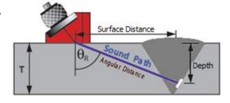
If a reflector came across the sound beam after it has reached and reflected off the backwall, the reflection is usually referred to as "second leg reflection". In this case, the
