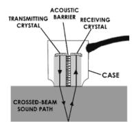
the element cannot start receiving reflected signals until the element has stopped ringing from its transmit function). Dual element transducers are very useful when making thickness measurements of thin materials and when inspecting for near surface defects. The two elements are angled towards each other to create a crossed-beam sound path in the test material.
