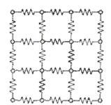
A mass on a spring has a single resonant frequency (natural frequency) determined by its spring constant k and its mass m. Within the elastic limit of any material, there is a linear relationship between the displacement of a particle and the force attempting to restore the particle to its equilibrium position.
