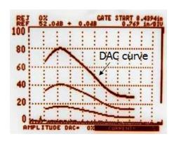
DAC will allow for loss in amplitude over material depth (time) to be represented graphically on the A-scan display. Because near field length and beam spread vary according to transducer size and frequency, and materials vary in attenuation and velocity, a <u>DAC curve must be established for each different situation</u>. DAC may be employed in both longitudinal and shear modes of operation as well as either contact or immersion inspection techniques.
