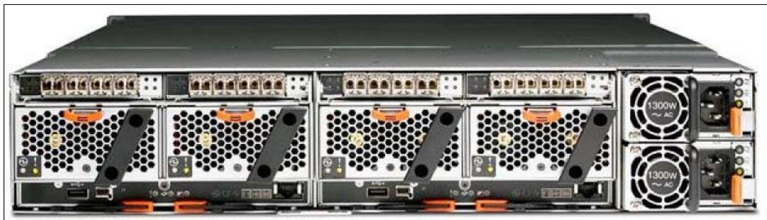
Figure 9 Rear view of FlashSystem V9000 storage enclosure
