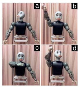
Figure 2. (a) Bandit pointing with its head; (b) straight-arm; (c), bentarm; and (d) and head+arm.
