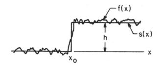
Fig. 4 One-dimensional edge fitting model [4].
