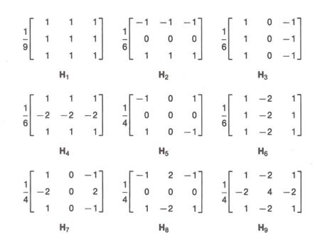
Fig. 3 Nine 3 by 3 impulse response arrays based on Chebyshev polynomial [4].
