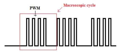
Figure 5, software level calibration of motor speed. PWM signal is sent to the motors during part of the time in the macroscopic cycle. The motors are actually repeating start and stop in each macroscopic cycle. This will cause the robot to move slower.
