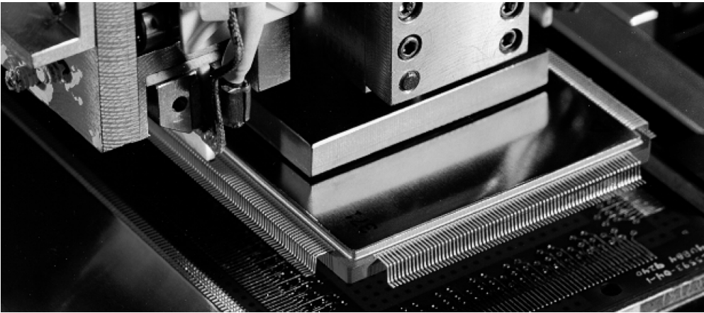
FIGURE 10.9 A robot assembles an electronic package onto a printed wiring board.
