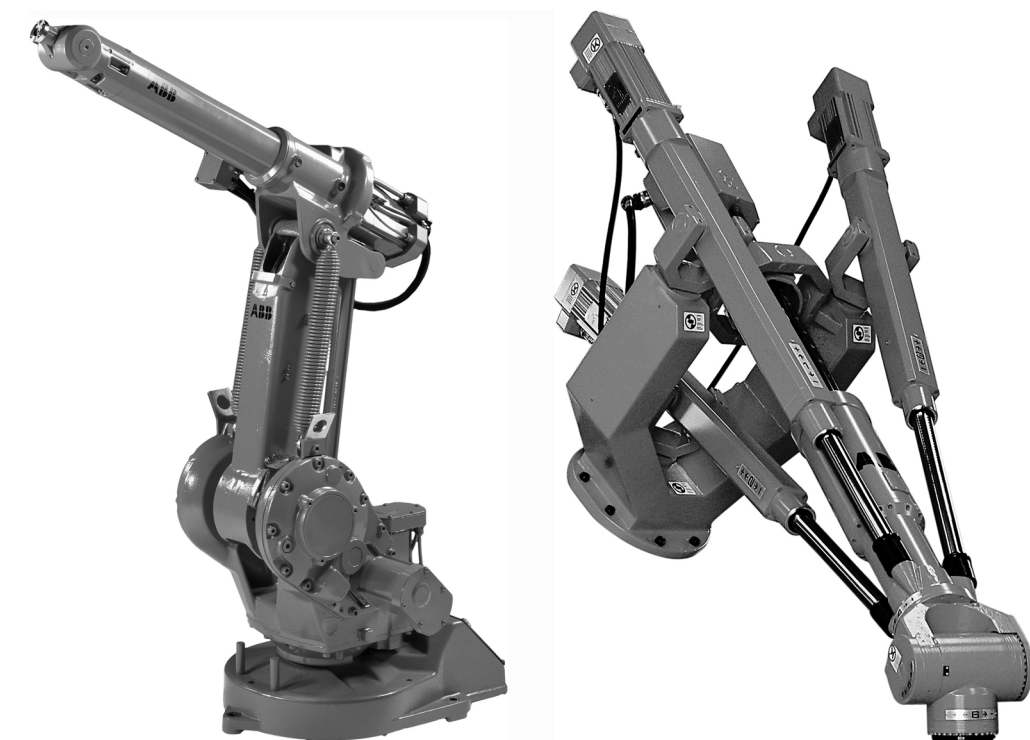
FIGURE 17.1 A serial manipulator (left), the ABB IRB1400, and a parallel manipulator (right), the ABB IRB940Tricept. (Photos courtesy of ABB Robotics.)
