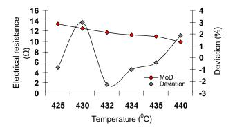
Figure 9. Variation of derived model predicted electrical resistance with melting temperature relative to its associated deviation from experimental results
