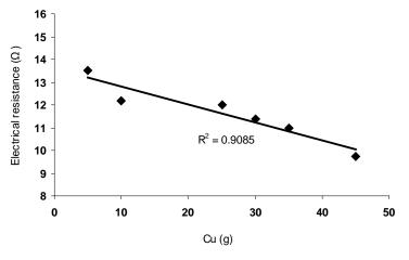
Figure 3. Coefficient of determination between Pb-Sb-Cu alloy electrical resistance and copper input concentration as obtained from experiment
