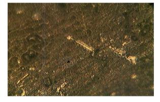
Figure 15. Microstructure of Pb-Sb matrix, 6.54%Cu x400
