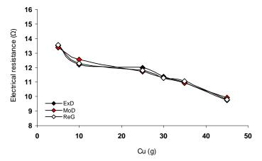
Figure 8. Comparison of Pb-Sb-Cu alloy electrical resistances (relative to copper input concentration) as obtained from experiment, derived model and regression model
