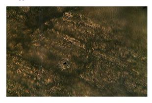
Figure 12. Microstructure of Pb-Sb matrix, 1.96%Cu x400
