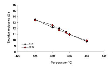
Figure 5. Comparison of Pb-Sb-Cu alloy electrical resistances (relative to melting temperature) as obtained from experiment and derived model
