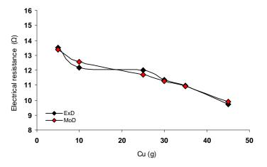
Figure 6. Comparison of Pb-Sb-Cu alloy electrical resistances (relative to copper input concentration) as obtained from experiment and derived model
