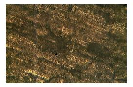
Figure 11. Microstructure of Pb-Sb matrix (Control) x400
