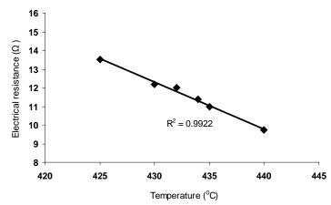
Figure 1. Coefficient of determination between Pb-Sb-Cu alloy electrical resistance and melting temperature as obtained from experiment
