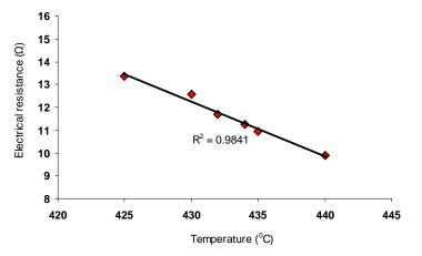
Figure 2. Coefficient of determination between Pb-Sb-Cu alloy electrical resistance and melting temperature as predicted by model
