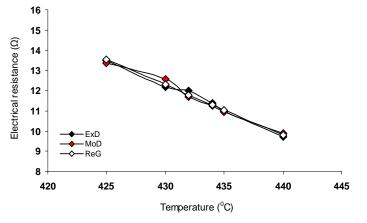
Figure 7. Comparison of Pb-Sb-Cu alloy electrical resistances (relative to melting temperature) as obtained from experiment, derived model and regression model
