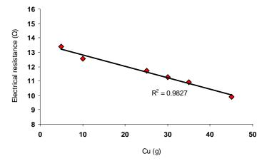
Figure 4. Coefficient of determination between Pb-Sb-Cu alloy electrical resistance and copper input concentration as predicted by model
