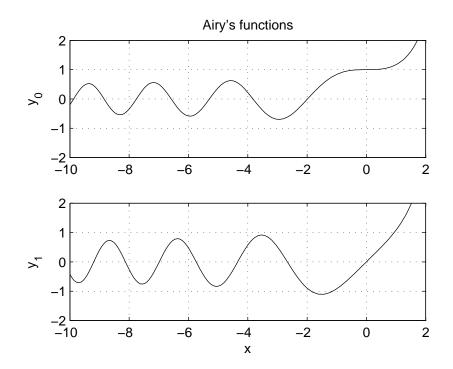
Figure 5.1: Numerical solution of Airy's equation.
