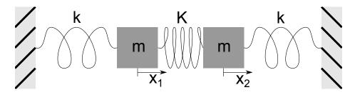
Figure 6.5: Coupled harmonic oscillators.
