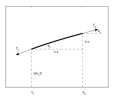
Figure 8.2: Derivation of the wave equation.
