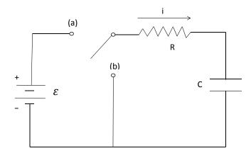
Figure 2.3: RC circuit diagram.
