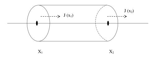
Figure 8.1: Derivation of the diffusion equation.
