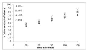
Figure 5. Effect of pH on efficiency of Colour removal for Fe-Fe Electrodes
