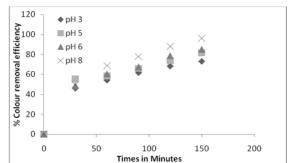
Figure 6. Effect of pH on efficiency of Colour removal for Al-Al Electrodes
