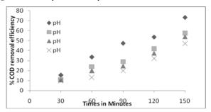
Figure 4. Effect of pH on efficiency of COD removal for Fe-Fe Electrodes
