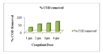
Figure 9. Effect of (Alum) coagulant dose on the COD removal efficiency
