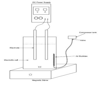
Figure 1. Electro coagulation Treatment
