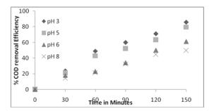
Figure 3. Effect of pH on efficiency of COD removal for Al-Al Electrodes
