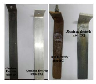
Figure 8. Electrodes before and after [EC]
