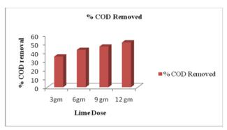
Figure 10. Effect of (Lime) coagulant dose on the COD removal Efficiency
