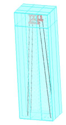
Figure 2. Meshing of semi submersible platform with 4 mooring lines
