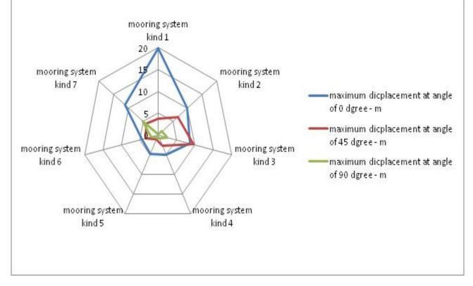
Figure 6. Semi-submersible platform Surge movement
