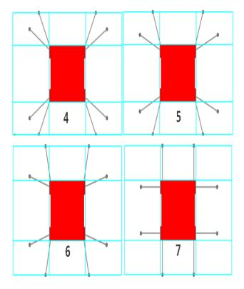
Figure 5. 4 kind of mooring system arrangement with 8 mooring lines
