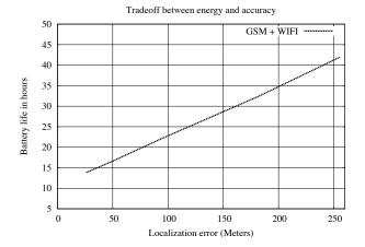
Figure 12: Energy accuracy tradeoff with proposed GSM + WiFi interpolation heuristic.
