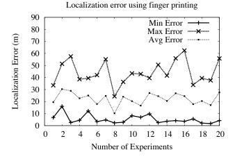
Figure 9: Minimum, Maximum, and average error based on localization using WiFi fingerprinting.
