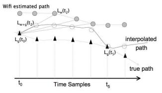
Figure 5: Interpolation between two localization schemes to achieve the advantages of both.
