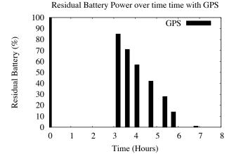
Figure 4: Energy consumption with GPS based localization for Nokia N95 phones.
