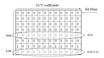
Figure 3. An example of bit plane encoding schema [9]
