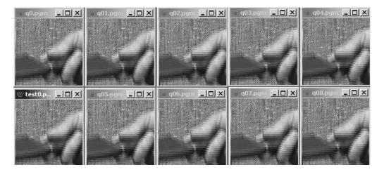
Figure 5. FGS effect on the 128x128, 8-bit grayscale picture In the figure, q0.pgm is the base plane, test0.pgm is the original picture. Pictures with name of q0x.pgm is the combination of base plane with the x bit planes from the most significant bit plane, in this case is 7.
