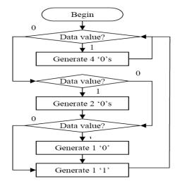
Figure 7. Golomb decoder algorithm (parameter m = 4)
