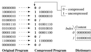
Figure 3. Bitstream compression using dictionary selection
