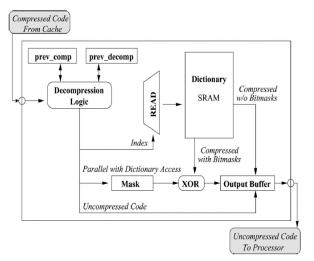
Figure 10. Decompression Engine
