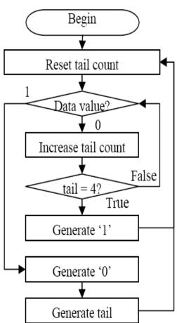
Figure 6. Golomb encoder algorithm (parameter m = 4)
