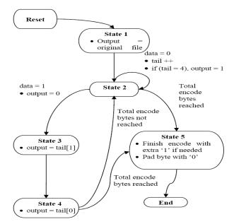
Figure 8. Golomb encoder algorithm on FPGA with Parameter m = 4
