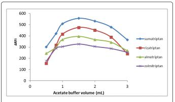
Figure 4: Acetate buffer volume effect (pH 3.5) on the reaction between the studied drugs (1  $\mu$ g/ mL) and Eosin (0.72 × 10<sup>-5</sup> M).
