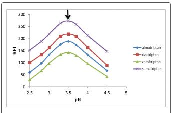
Figure 3: pH effect of 0.2 M acetate buffer on the reaction of the studied drugs (1µg/mL) with Eosin (0.72  $\times$  10<sup>-5</sup> M).
