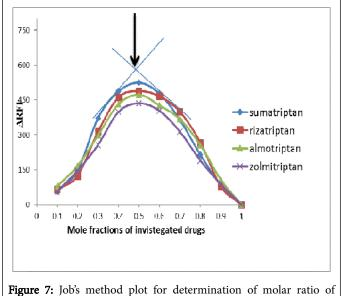
**Figure 7:** Job's method plot for determination of molar ratio of studied drugs and Eosin Y using  $0.72 \times 10^{-5}$  M equimolar solutions.
