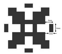
Fig.3: unit patch of FSS with modified design I
