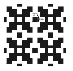
Fig4: FSS showing four unit cell with modified design.
