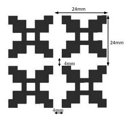
Fig2: FSS showing four unit cell and spacing between them.
