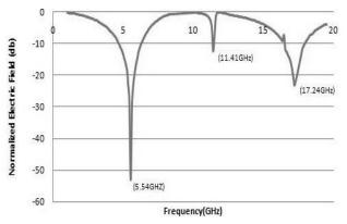
Fig 7: Normalized Transmitted Electric Field vs. Frequency for the First Design.
