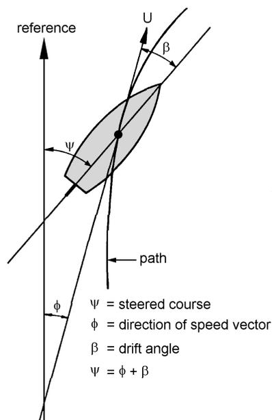
Figure 4.1: Definition of Course and Drift Angle
