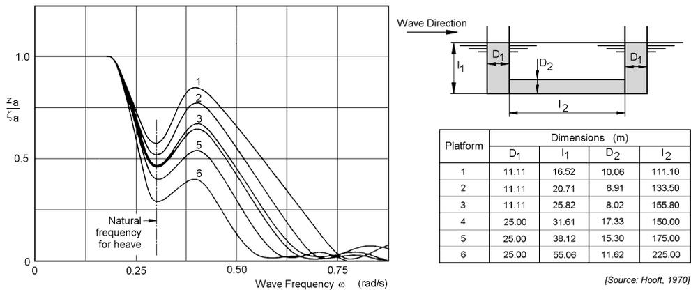
Figure 3.15: Heave Responses of Semi-Submersible Platforms in Waves
