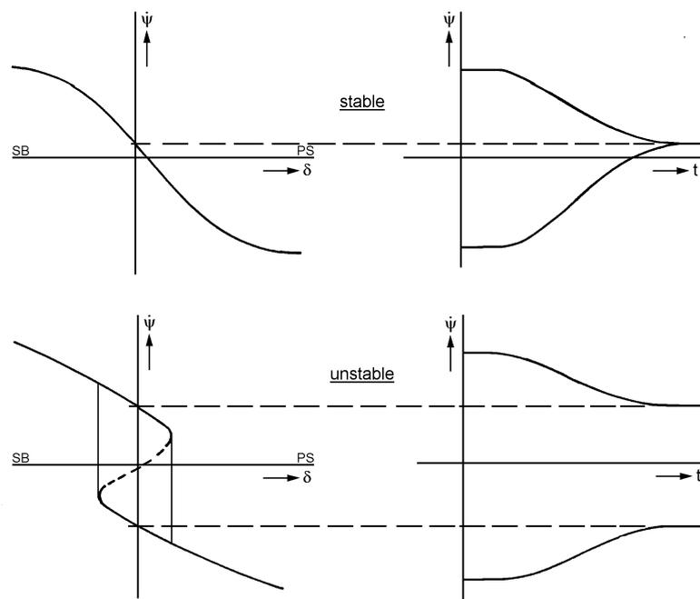
Figure 4.17: Results of a Pull-Out Test for a Stable and an Unstable Ship
