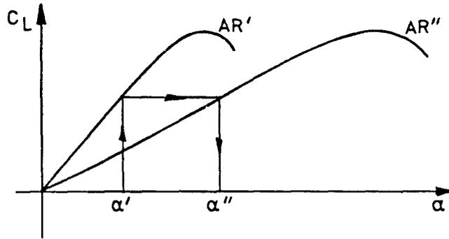
Figure 4.6: Aspect Ratio Transformation of Lift Coefficients
