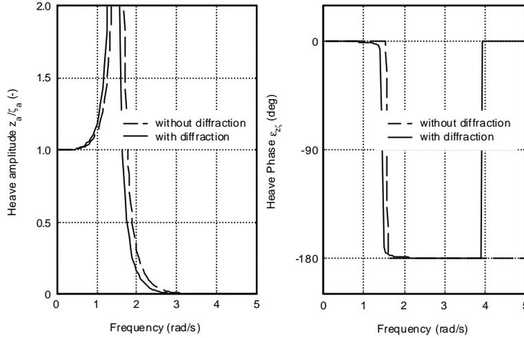
Figure 3.11: Heave Motions of a Vertical Cylinder
