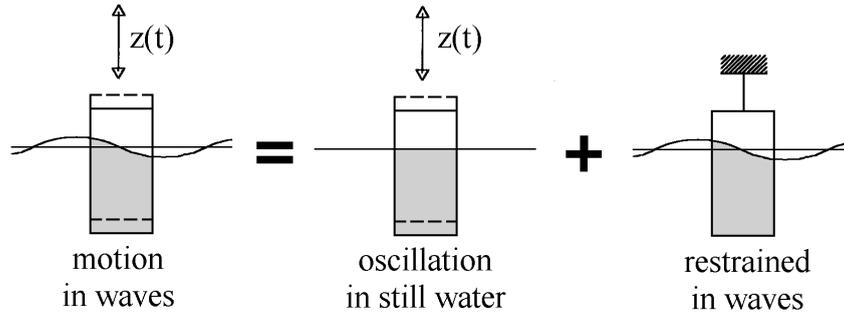
Figure 3.7: Superposition of Hydromechanical and Wave Loads
