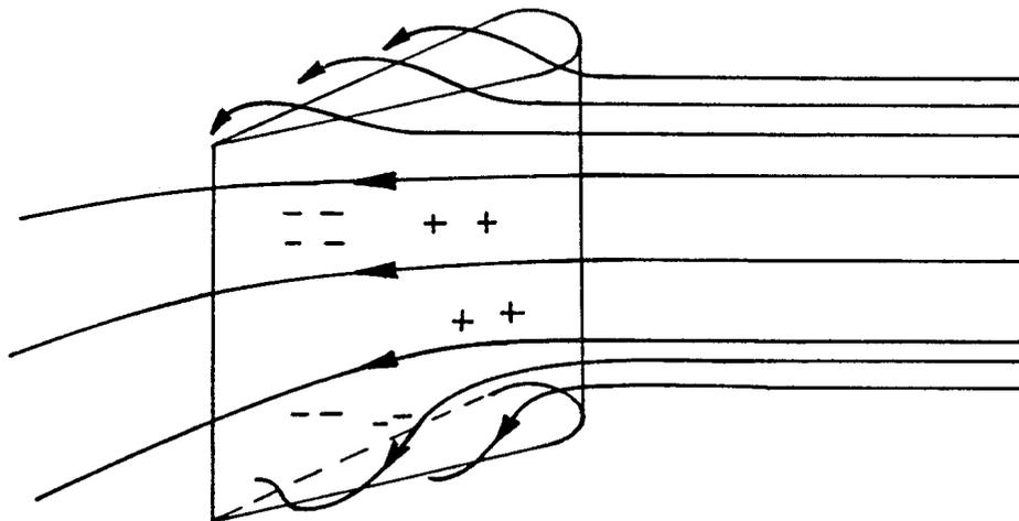
Figure 4.5: Flow Around Corners of a Lifting Surface
