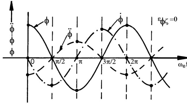
Figure 3.5: Displacement, Acceleration and Velocity
