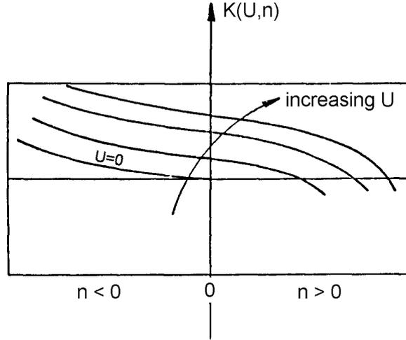
Figure 4.30: Breaking Force as Function of Forward Speed and Propeller Rate
