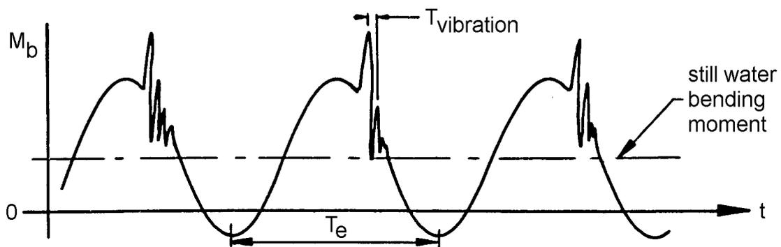
Figure 1.2: Amidships Vertical Bending Moments During Slamming
