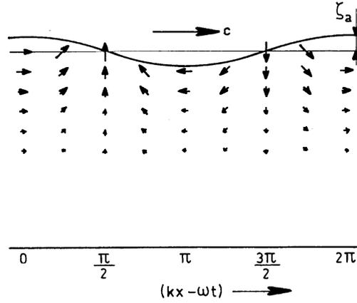
Figure 2.2: Velocity Field in a Deep Water Wave
