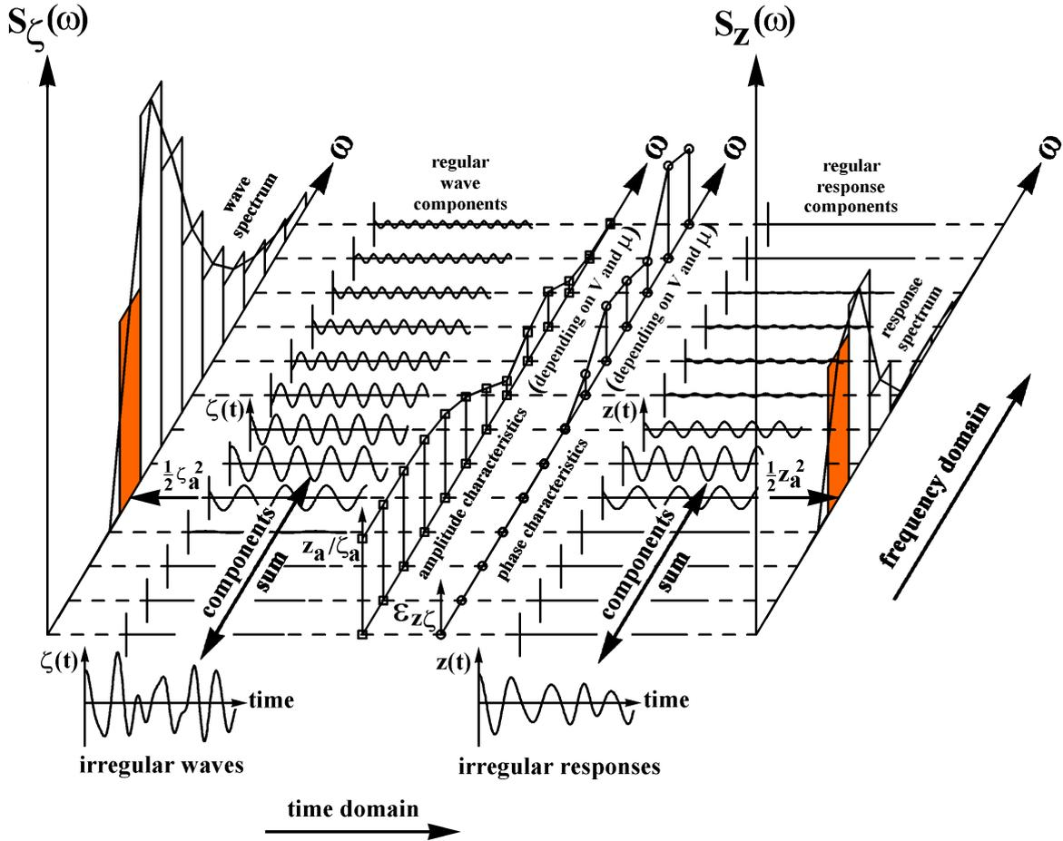
Figure 3.16: Principle of Transfer of Waves into Responses
