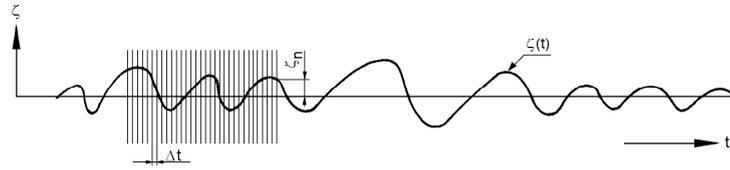
Figure 2.8: Registration and Sampling of a Wave
