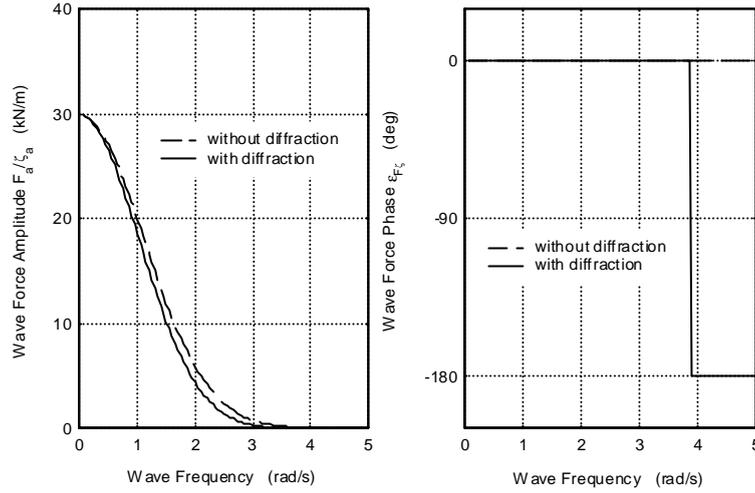
Figure 3.10: Vertical Wave Force on a Vertical Cylinder
