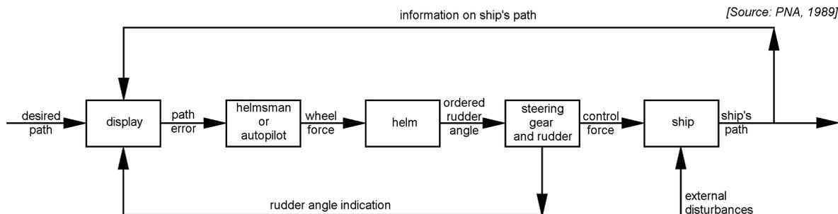
Figure 4.8: Closed-Loop Control System of Ship Controllability
