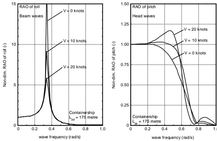
Figure 3.13: RAO's of Roll and Pitch of a Containership
