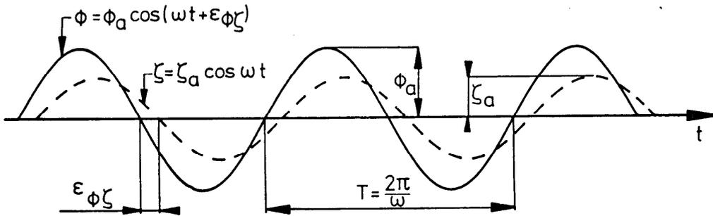
Figure 3.4: Harmonic Wave and Roll Signal
