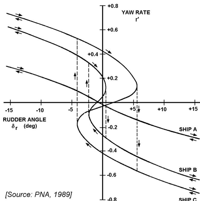
Figure 4.20: Steady Turning Rate Versus Rudder Angle
