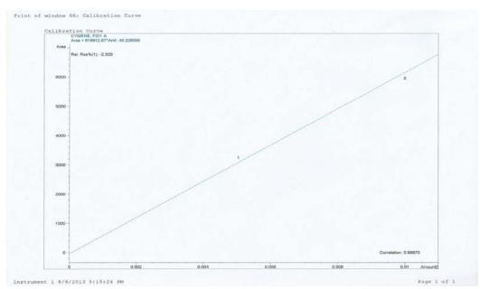
Figure 3. calibration curve of cymene
