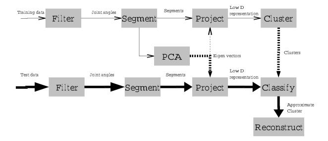
**Fig. 3.** Components of our system. Thin lines represent the flow of data in the training phase. Dark lines represent the flow of data in the testing phase. Dotted lines represent the use of previously computed data.
