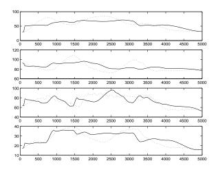
**Fig. 9.** Reconstruction of an entire movement composed of multiple segments. Each subplot shows one angle as a function of time. The solid line shows the original movement, the dotted line the reconstruction.
