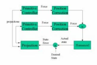
**Fig. 12.** The controllers model. The Primitive Controller is an individual controller for each primitive. The Position Correction module corrects for changes in the location of the center of the stroke. In this work, the Humanoid is modeled by Adonis. The Projection Module projects the errors back onto the eigenmovement space.
