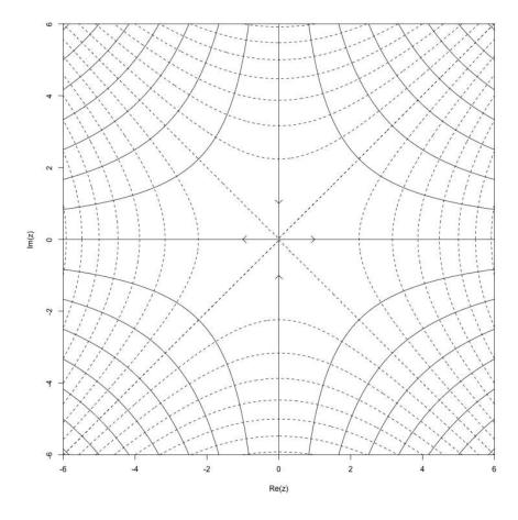
Figure 7: Potential flow on the complex plane: field corresponding to the function  $(z) = z^2$ . Solid lines represent streamlines and dotted lines represent equipotentials; these intersect at right angles. Note stagnation point at the origin
