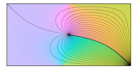
Figure 9: Potential flow in a rectangle of aspect ratio 2: source and sink of equal strength. Colour scheme as in figure 8. Note the dividing streamline which terminates in a stagnation point on the rectangle boundary
