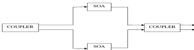
Fig 3.1 Optical logic using MZI switch
