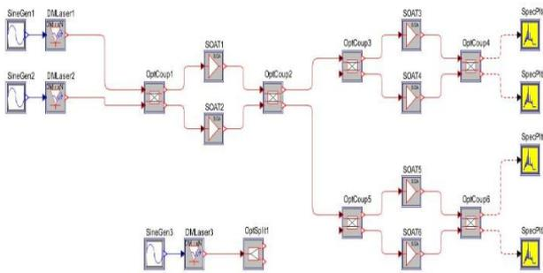
Fig 3.3 Schematic Diagram of Multiplexer (A = '1', B = '0')
