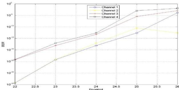
Fig 4.3 BER versus power control signal with dispersion
