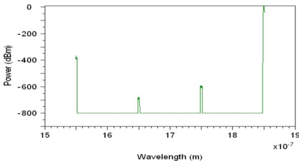
Fig 3.6 Wavelength spectrum of A = '1' & B = '1', EN = '1'
