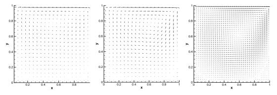
Fig. 4.2. Velocity field for Example 4.2. From left to right: Re = 1, 100 and 400.
