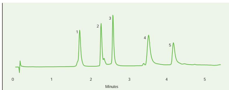
Figure 24. Column: C_{18} , 3 \mu\text{m} 4.6 x 50 mm (VYDAC® 238TP3405). Flow rate: 4.0 ml/min. Eluent: Gradient from 20–45% ACN in aqueous 0.1% TFA in 4 min. Sample: protein standards. (1) ribonuclease, (2) insulin, (3) cytochrome c, (4) BSA and (5) myoglobin.
