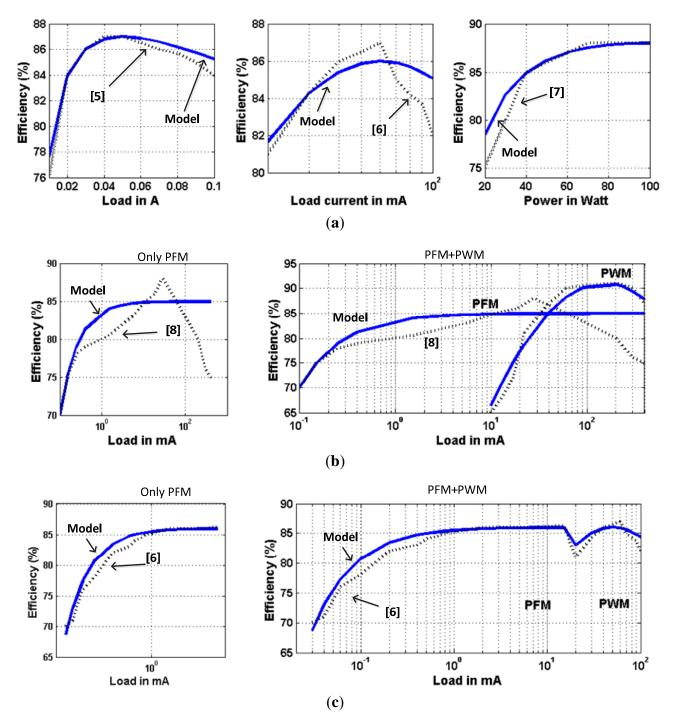
To further illustrate the usefulness of the model, we also compared it with the schemes where both PFM and PWM schemes are employed. This is often done to increase the range of load a converter can support. Figure 4b,c shows the results of comparison of the model with efficiencies reported in [6] and [8]. The model accurately predicts the behavior of such converters. There can be several other combinations in which the model can be used. For example, the model can be used for a segmented
