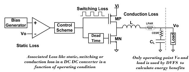
Figure 2. Loss mechanisms inside a typical switching DC-DC converter.
