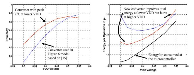
In addition to supporting the co-design of embedded DC-DC converters, our model can enable higher level comparisons of power management techniques that apply to multiple blocks. The next example illustrates the application of our model to two different power management strategies.
