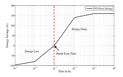
Figure 10. Energy Savings with rate of Voltage Scaling.
