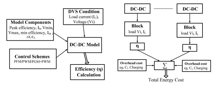
Figure 1 shows the structure of the proposed model, which is broken into two parts. First, a model of inductor based DC-DC converters (Figure 1a) takes the operating condition of a workload as an input, which includes peak efficiency, load at which the peak occurs, minimum efficiency, maximum and minimum output voltages, settling time, and the decoupling capacitance of the DC-DC converter, and generates an efficiency calculation. In order to capture the dynamic load condition of the converter
