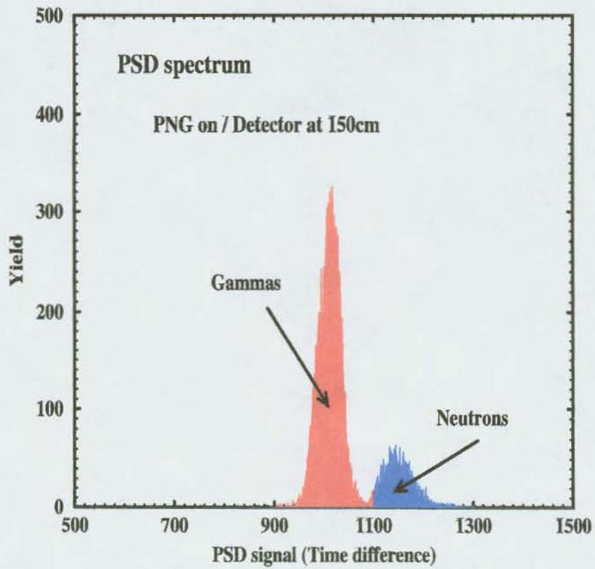
Figure 2: A pulse shape discrimination spectrum. This is a time spectrum showing the difference between a pulse start time and the cross over after differentiation
