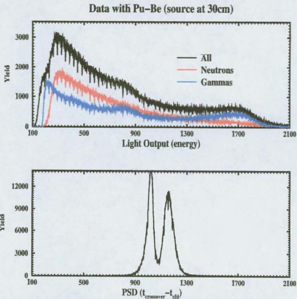
Figure 3: The light out put of the PD neutron detector for all signals and neutron and  $\gamma$  gated signals. The PSD pulse is shown in the lower part.
