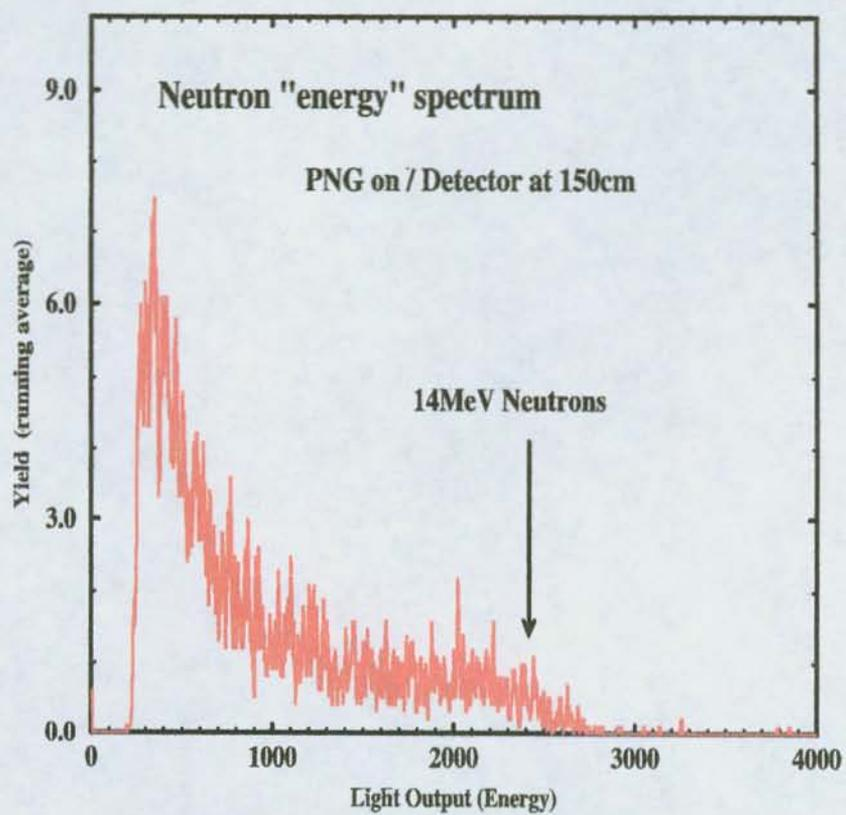
Figure 4: The light output of the PD neutron detector for signals gated on neutrons in the PSD pulse.
