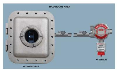
Instead of having both the sensor and the controller rated explosionproof (XP), explosionproof sensor housings are sometimes used with general purpose (GP) controllers that are located in non-hazardous locations.
