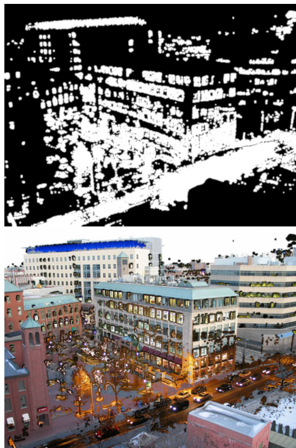
Figure 5: Importance mask used for blending gradients and Result of simple linear blend of pixel intensities showing artifacts.
