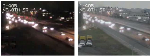
Figure 2: Enhanced traffic video. A low quality nighttime image, and the final output of our algorithm (Please see the video submission).
