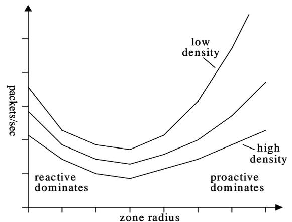
Figure 8: ZRP traffic per node (schematic)
