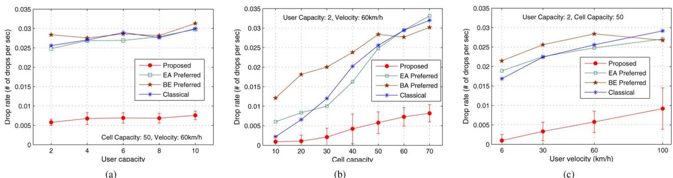
Fig. 8. Drop rate: (a) user capacity, (b) cell occupancy, and (c) user velocity.
