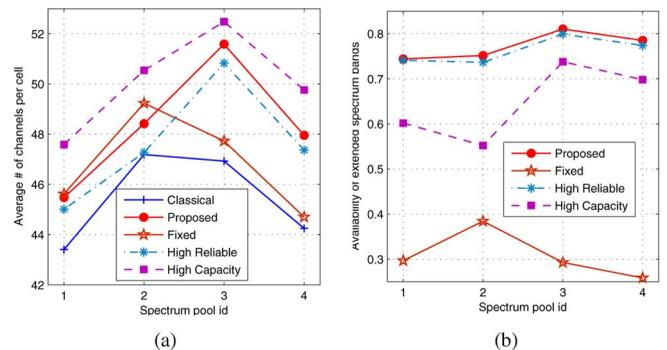
Fig. 6. Intercell resource allocation: (a) total available channels and (b) availability in extended spectrum bands.
