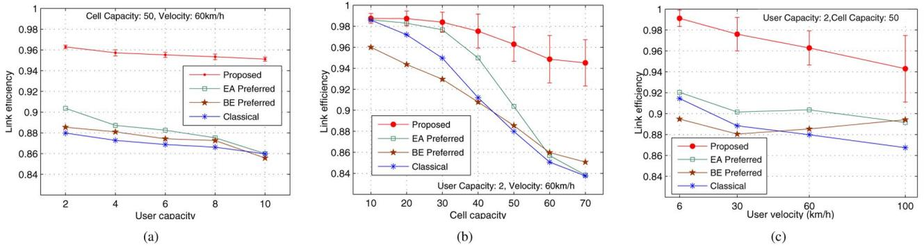
Fig. 9. Link efficiency: (a) user capacity, (b) cell occupancy, and (c) user velocity.
