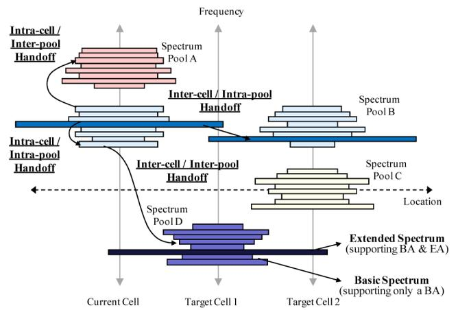
Fig. 2. Different handoff types in CR networks.
