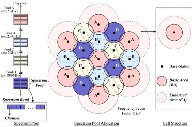
Fig. 1. Spectrum pool-based CR network architecture.
