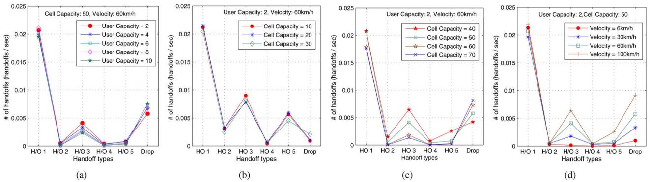
Fig. 7. Handoff types: (a) user capacity, (b) lower cell occupancy, (c) higher cell occupancy, and (d) user velocity.
