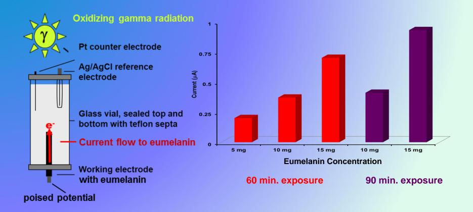
Irradiated eumelanin was able to allow electrons to flow through it. The more eumelanin in the electrodes and the longer the exposure time, the more current was produced.
