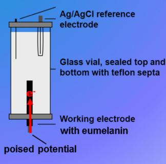
In order to test the hypothesis that radiation turns eumelanin into a "bottomless pit" for electrons we set up the following experiment. With eumelanin isolated from the surface of fungal cells we constructed an electrode and placed it next to a radiation source. With the electrodes connected to a potentiostat, a potential was applied to the eumelanin electrode. Next we turned on the radiation. If gamma radiation oxidized the eumelanin an electric current would flow.
