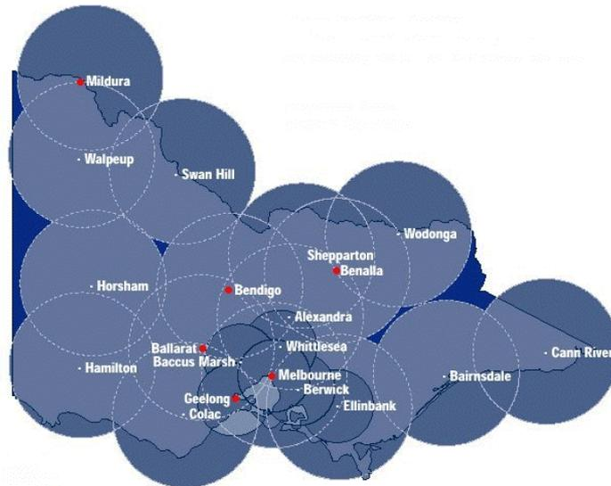
**Figure 5:** GPSNet Victoria. Note large circles 100km radius, small circles 50km radius.
