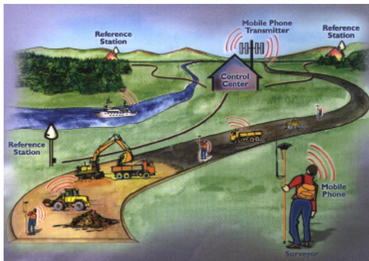
**Figure 6:** Trimble's Virtual Reference Station concept.
