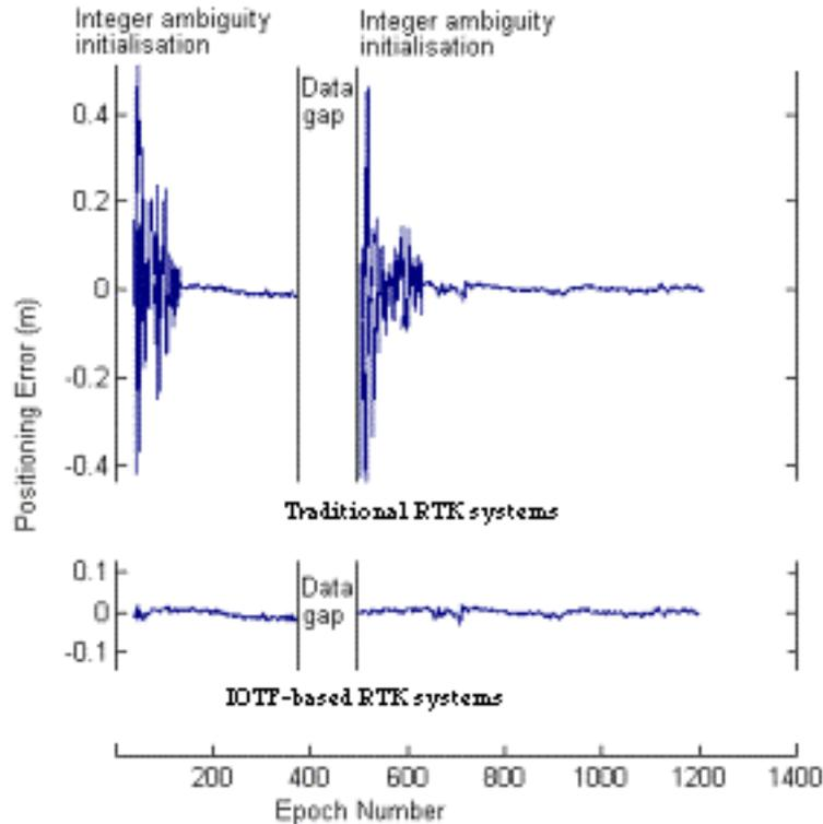
**Figure 2:** Comparison of RTK performance using standard multi-epoch OTF-AR techniques and the instantaneous OTF-AR technique. Note the 'dead' time (when accuracy is degraded) during which AR is being undertaken in upper plot, compared to lower plot for IOTF-AR.
