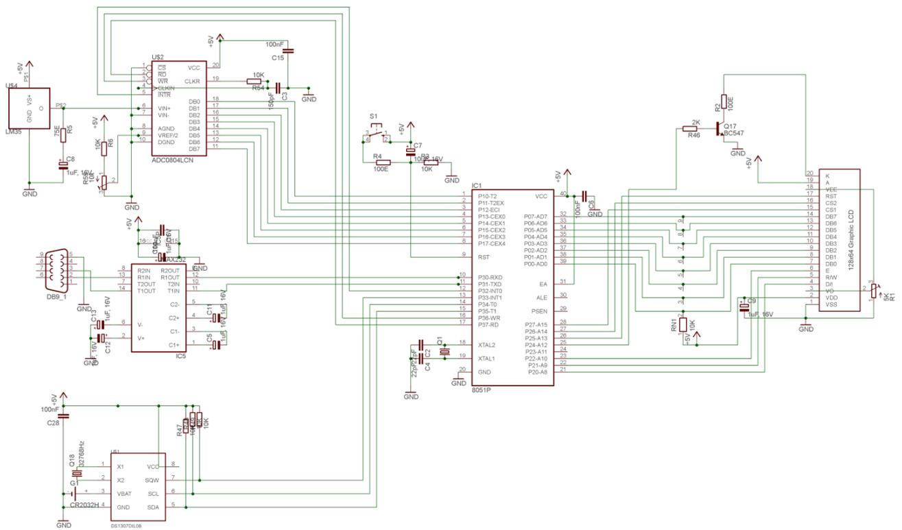
**Fig 3. Complete schematic diagram for the proposed system edited in EAGLE PCB Layout Editor**
