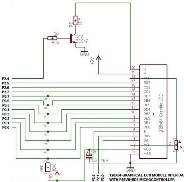
Fig 6. Schematic sub-block-3
