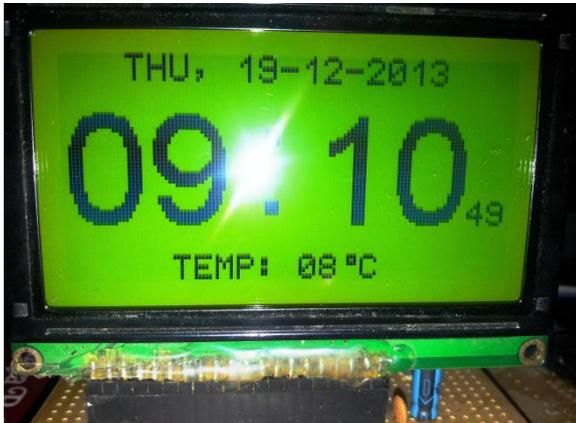
**Fig 4. Graphical LCD panel showing the day, date, time and temperature.**
