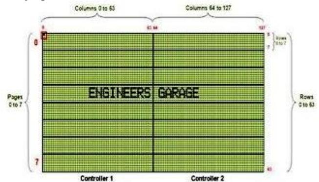
Fig 1. A 128x64 Graphical LCD arrangement.
