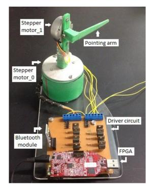
Figure 1. Physical setup of the BlueSteps system
