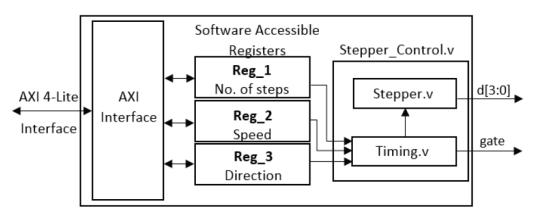
Figure 4. Block Diagram of the User\_Logic.v
