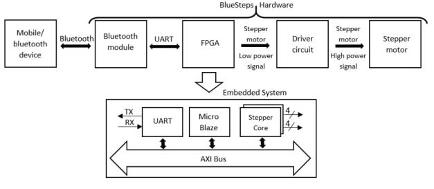
Figure 2. Block Diagram of the BlueSteps system
