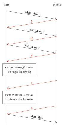
Figure 5. One cycle of dynamic communication between MB and Mobile phone. The messages shown in the diagram will cause stepper motor 0 to do 10 steps clockwise and stepper motor 1 to do 10 steps anticlockwise
