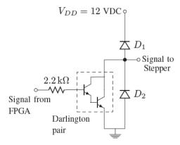
Figure 6. Driver circuit schematic
