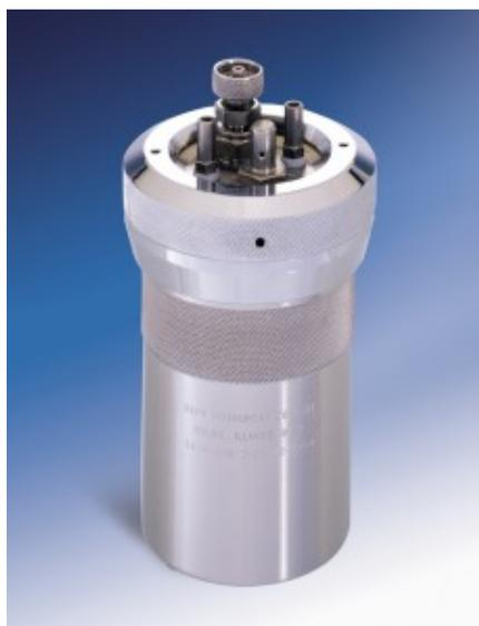
**Figure 1:** A Parr<sup>TM</sup> Model 1108 Oxygen Combustion Vessel<sup>®</sup>, as used in this experiment.
