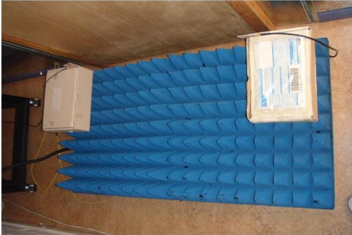
**Figure 12-The Group Delay measurement setup for Antipodal Vivaldi antenna in Chase group Lab at Chalmers**
