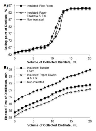
**Figure 3.** Data for the separation of a 50%  $(\nu/\nu)$  methanol and 1propanol mixture under similar conditions with a Vigreux fractionating column that was either non-insulated or insulated with either tubular polyethylene foam or paper towels and aluminum foil, respectively. A) Fractional distillation plots of boiling point versus volume of collected distillate. B) Plots of elapsed time of distillation versus volume of collected distillate
