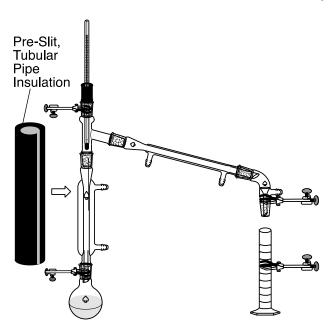
Figure 1. Schematic for employing pre-slit, tubular pipe insulation with a fractional distillation apparatus
