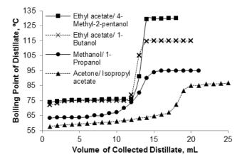
**Figure 2.** Example student fractional distillation plots for the separation of the four different binary mixtures employed for this experiment. These plots were selected from those submitted upon request at the end of the semester
