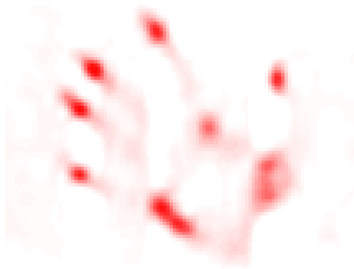
Figure 2.1: The SmartSkin touchpad returns an image of the distance from the touchpad to the hand.
