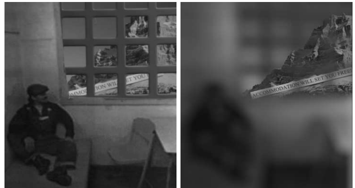
Figure 1: The “pinhole prison”: occluded portions of the background scene are not visible using a pinhole camera (left). Using a finite aperture and a lens, however, allows one to see past the occlusion (right). A similar effect can be seen in the scene in Figure 8.
